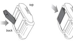
5. The OnSite will automatically run a self-test when the battery is inserted. Press the Shock button when instructed. When the self-test is over, the OnSite will report the result, and tell you to push the green On/Off button in case of an emergency. (Do not push the green button unless this is an actual emergency.) Then the OnSite will turn off and go to standby mode. The green Ready light will be blinking to show the OnSite is ready for use.\*
